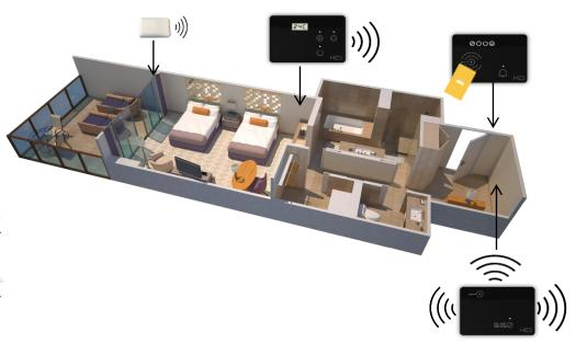
Through wireless technology, the devices communicate with each other and with the "Suite 224" software at the reception desk, without cables or data network, managing the hotel in real time, through the software and also the innovative APP "SMART".
